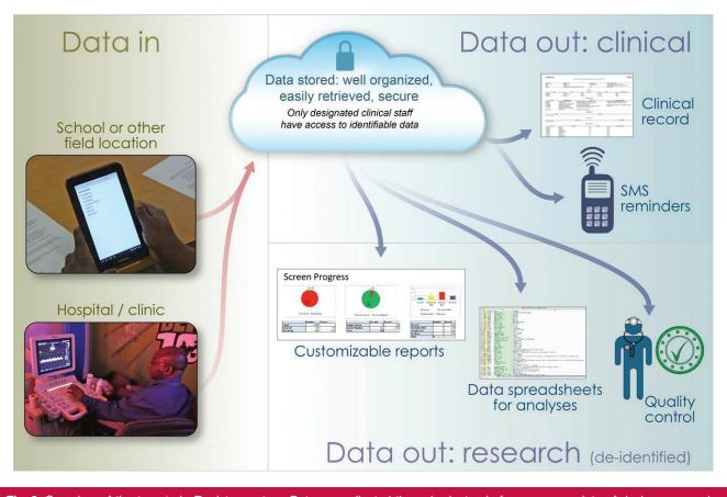
Fig. 3. Overview of the targeted eRegister system. Data are collected through electronic forms on a variety of devices, securely managed in the cloud, and made accessible to multiple users for varying clinical care and clinical research purposes.
